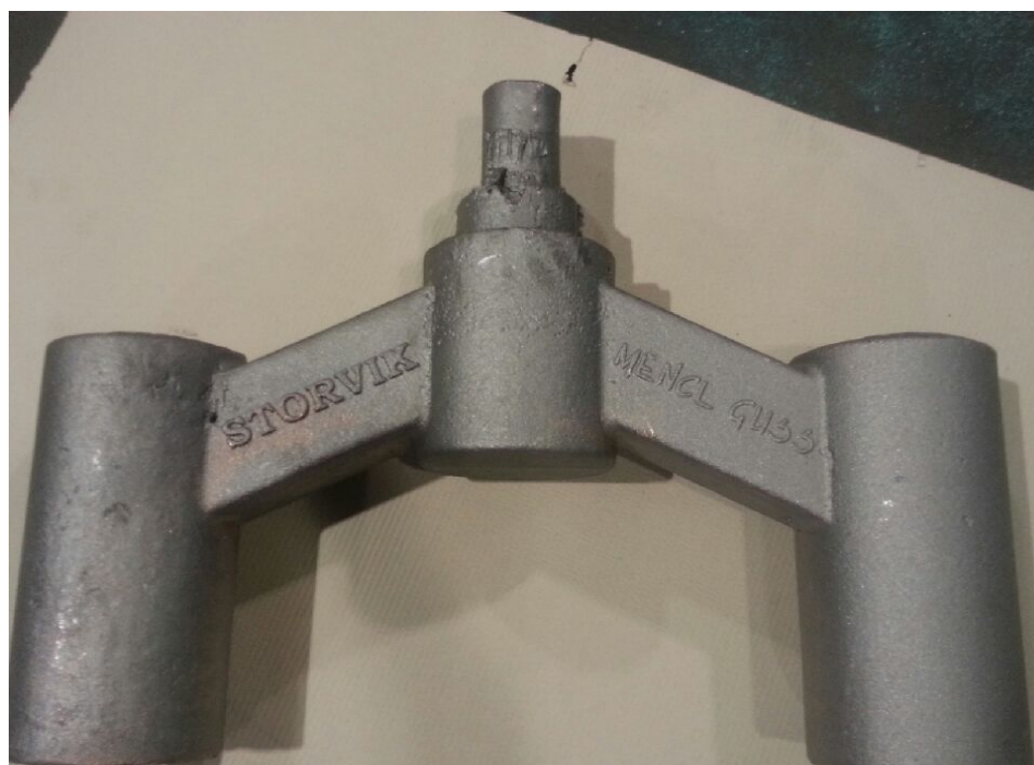
Figure 8. Storvik HC Anode yoke with Cu core.
