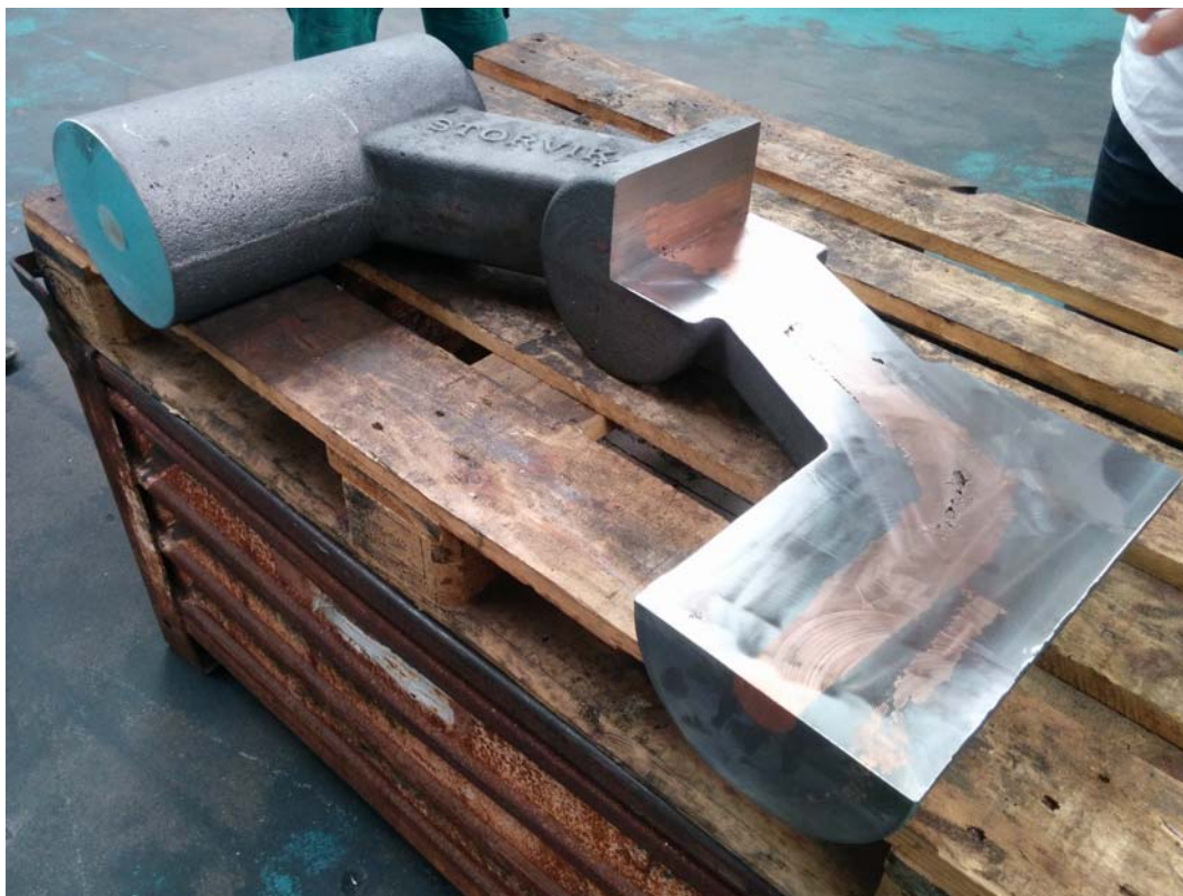
Figure 9. Machined cross section of anode yoke.
