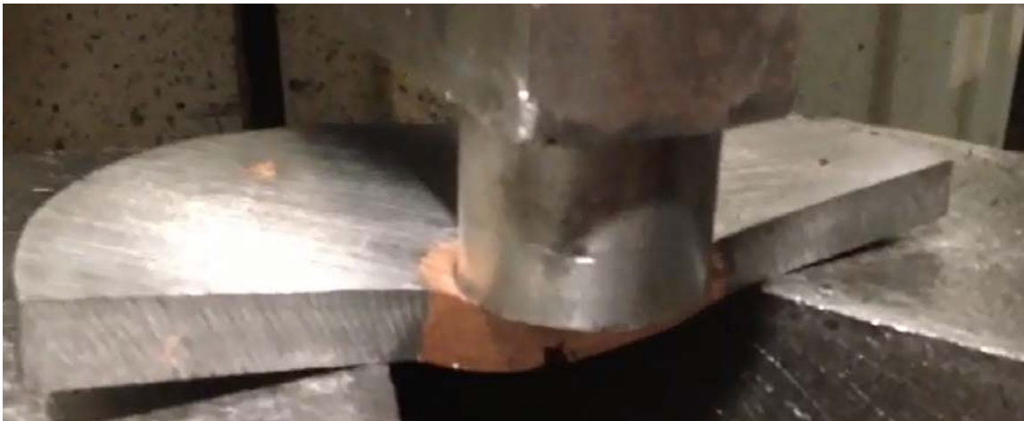
Figure 6. Destructive testing of molecular bond.
